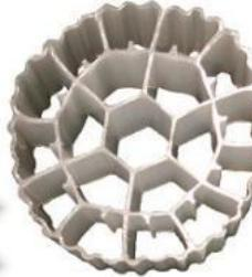
Different kind of bio filters such as trickling, submerged and MMBR have designed and produced in technoaaby group. Biofilteraion is suitable way for removing ammonia and oxidized it to nitrate. Biofiltration is a good choice for increasing water production capacity in fish farming. High specific surface area, resistant materials of media and anti-clogging design is advantages of technoaaby bio filters.
